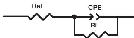
Figure 4: EEC model used to fit EIS data recorded CS in absence and presence of the inhibitor.
